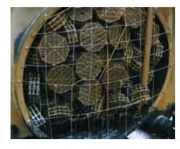
The initial result of the TVT-BIO 32 Bioreactor is the reduction of the ice cover in the lagoon by two thirds, and odor removal (Oxygen transfer) started even
